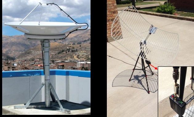
“Professional” (Left) & Low Cost (Right) HRIT/EMWIN Antennas
