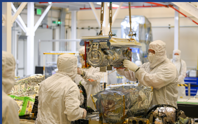
Engineers integrate the nation's first coronagraph on the NOAA GOES-U satellite. Image Credit: Lockheed Martin
