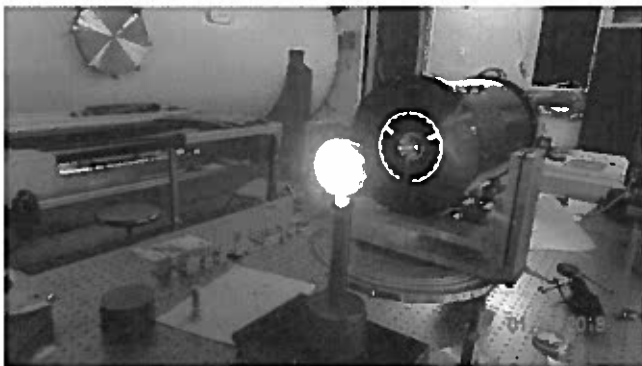
Figure 1. CCOR instrument optical test bed initial illumination test
