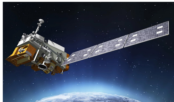
NOAA-20, 1 out of 2 satellites in the Joint Polar Satellite System (JPSS). The “polar” in Joint Polar Satellite System means these satellites orbit the North and South Poles. As JPSS orbits the poles, the Earth spins underneath, allowing the satellites to observe all of Earth’s surface, oceans, and atmosphere below twice in one day.
