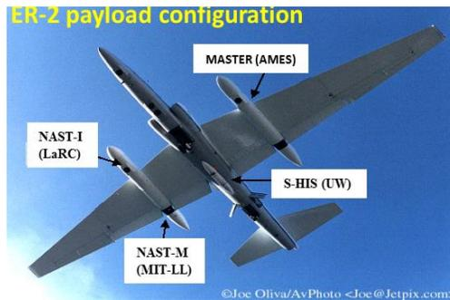
*The NASA ER-2 research aircraft equipped with NAST-I, NAST-M, S-HIS and MASTER*
