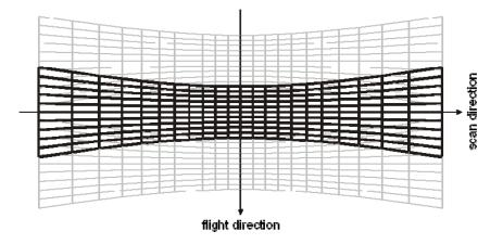
Three consecutive MODIS scans each consist of ten 1km lines. Due to the panoramic "bow tie" effect, the scans are partially overlapping at off Nadir angles. The first and third scans are represented by the light grey grids, while the second scan is shown in black.
